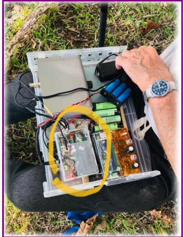
SWR bridge with LED indicators, and my 2 radios
