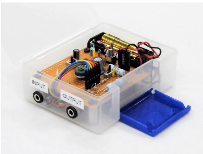
Fig 1. Complete audio amplifier using an LM386 IC chip
