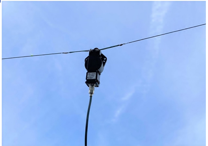
Figure 3. Dipole antenna using a balun
