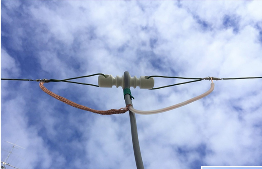
Figure 2. Dipole antenna without a balun
