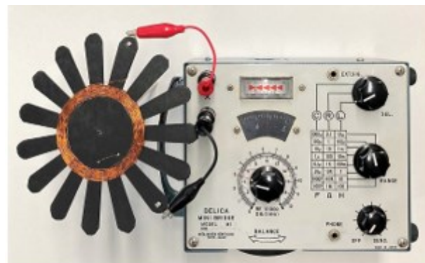
(b) Double-skip winding Figure 4. Measuring inductance
