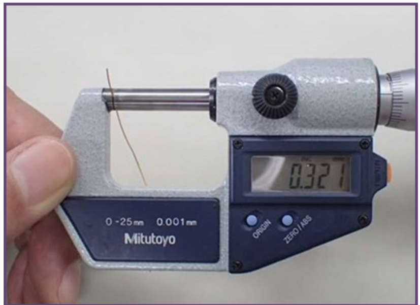
Figure 2. Measurement of the enameled wire diameter
