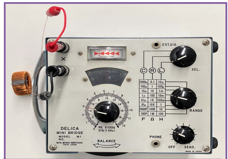
Figure 8. Measurement of inductor wound on a toroidal core
