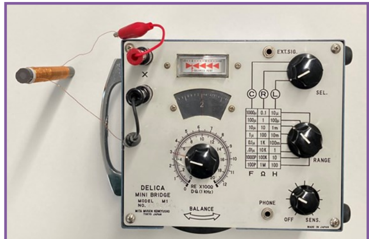
Figure 7. Measurement of inductance on a ferrite rod inductor
